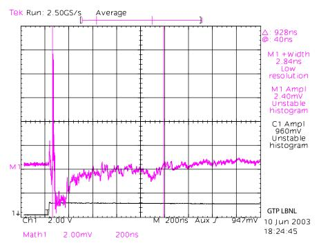
Ch1:Input pulse to twisted pair. (from outermost layer of spool) M1:Cross-talk signal within about 160 meters of the end of the cable.
