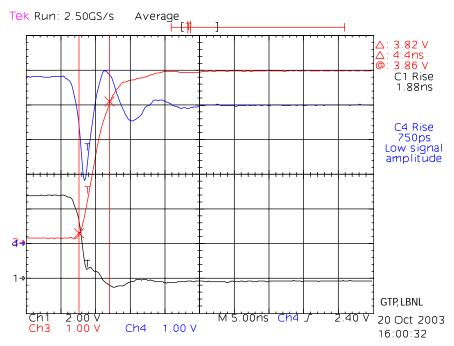
Ch1: '14 output. Ch3: FET Gate. Ch4: H81 Base. 47pF || 4.7K from '14 output to H81 Base. Measured with Active Probes
