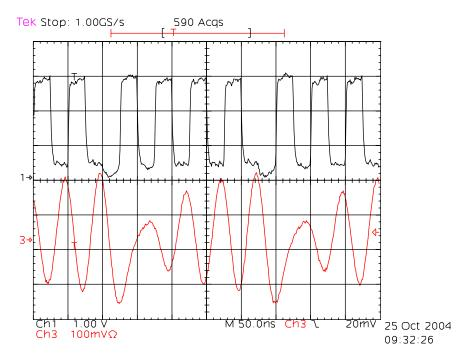
Ch1: Oscillator output pin Ch3: Filtered clk monitor test point.
