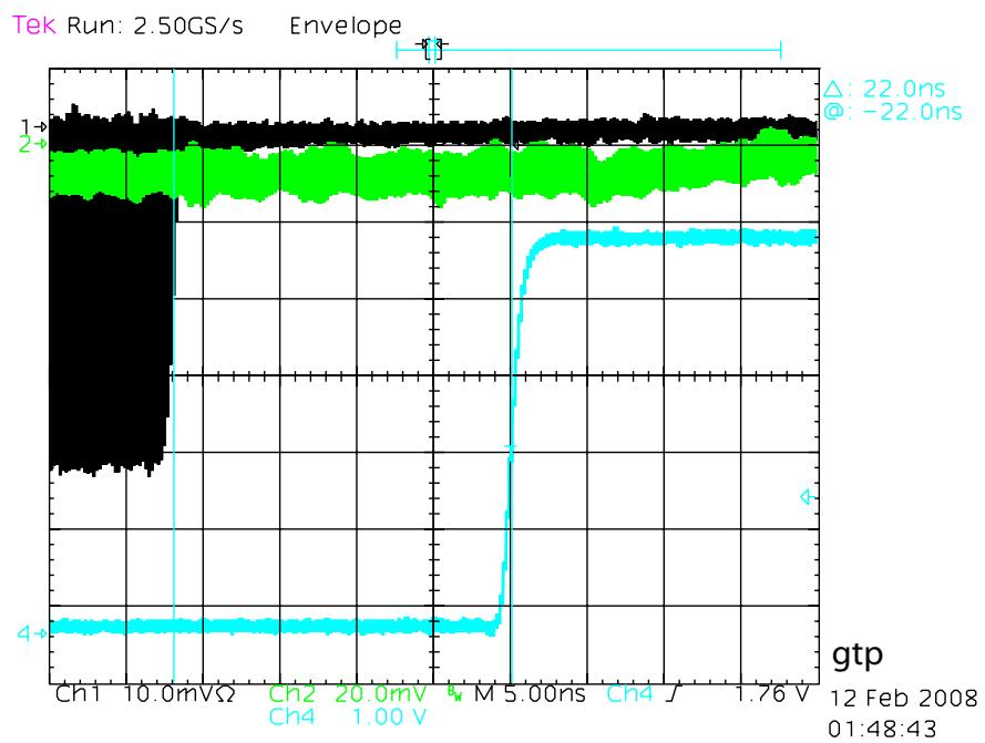
Input to Trigger minimum delay ~20ns (less calibration error)
