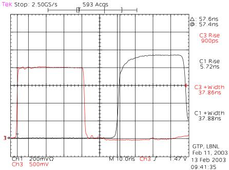
Square wave input to low-loss PCB delay line.
