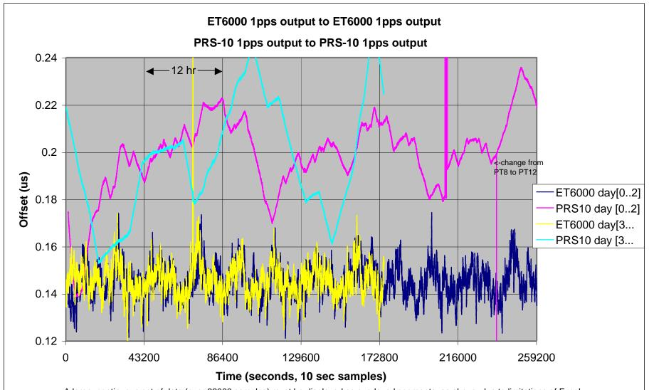
A large, continuous set of data (over 32000 samples) must be displayed as overlayed segments, as above, due to limitations of Excel. For convenience, the overlay period used here is three days = 25920 samples.
